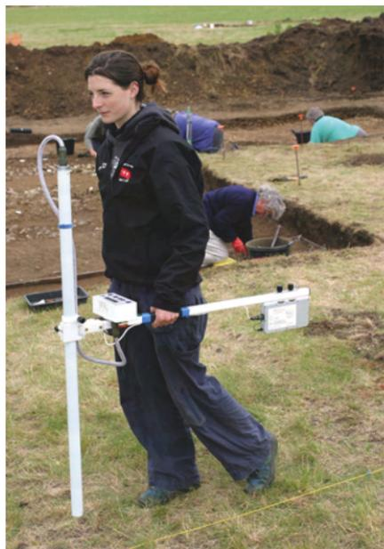
**Figure 2** This field researcher is using a Grad601 flux-gate gradiometer at an archeological-dig site (courtesy Bartington).
